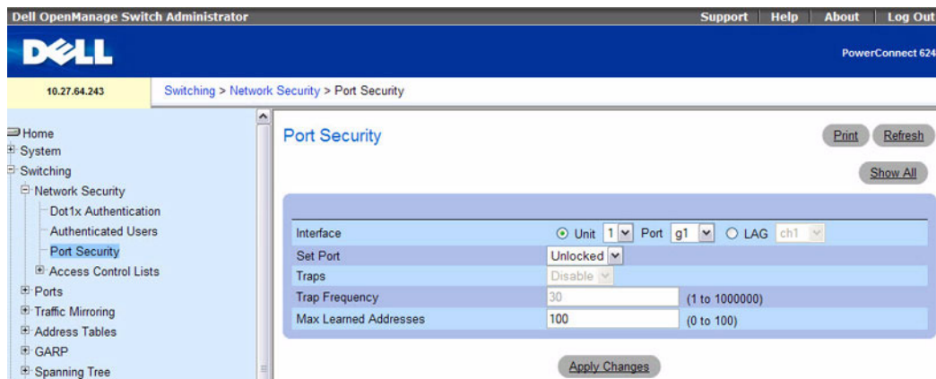
Figure 7-4. Network Security Port Security
